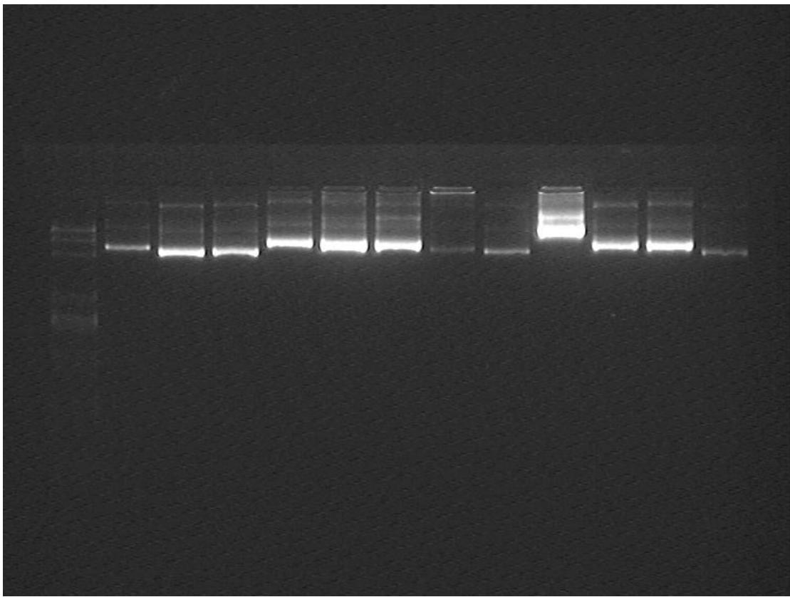
Causing the CI+1-4H samples are not very good, we do electrophoresis again: Agarose 2%.
