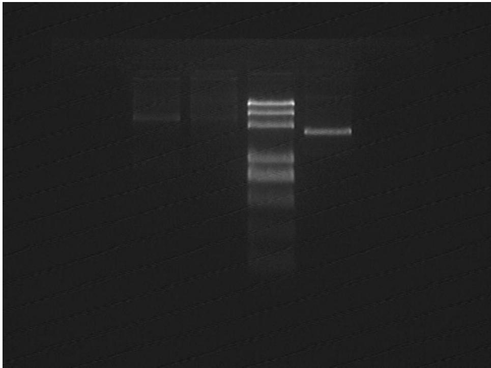
Result reveals that the double-digestion failed. The double-digested fragments can't be identified out in electrophoresis causing the concentration of plasmids in this enzymatic digestion system is too low.
