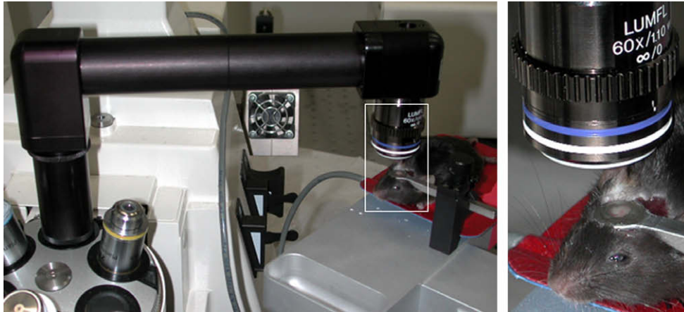
Fig. 1. Optical Imaging in vivo of the mouse parietal cortex. Left panel shows the objective inverter attached to a Zeiss LSM 510 multiphoton microscope positioning the 60× 1.1 NA water immersion objective above the mouse parietal cortex. Right panel is a higher magnification of the stainless steel ring holder that is glued to the skull and immobilizes the brain. The center ring has been filled with 2% agarose (Sigma type VII) and sealed from above with a glass coverslip (#0). This essentially eliminates motion artifacts due to breathing when the hole in the cranium is less than 1–2 mm in diameter. The red heating pad is maintained at 37 °C.
