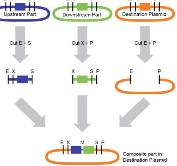
Start with two BioBrick parts and a BioBrick destination plasmid. The destination plasmid contains a toxic gene, ccdB, in the BioBrick cloning site and a different antibiotic resistance marker to the upstream and downstream parts.
