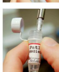
You will need three PCR tubes, one for the digest of the upstream part, one for the downstream part, and one for the destination plasmid. You should label each tube (for example, U, D, P, for upstream part, downstream part, and destination plasmid respectively).
